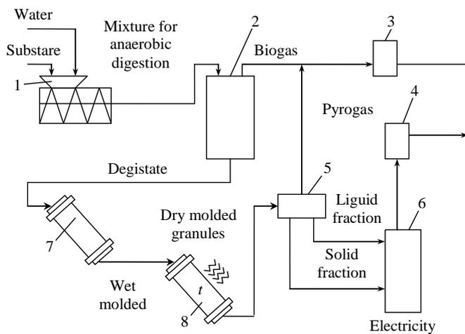
Fig. 1. General structural scheme of cogeneration complex of deep digestate processing: screw mixer (1); reactor-methanogenic (2); gas generator (3); electric generator on black oil (4); pyrolysis furnace (5); module for the production of heating oil (a substitute for fuel oil) (6); drum granulator (7); drum dryer (8)
