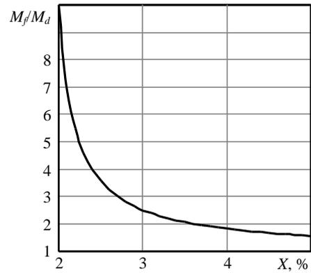
Fig. 2. Dependence of the ratio of water discharge  $M_f/M_d$  on saline content of boiling brine  $X_b$  with salinity of sea water  $X_f = 1.8\%$
