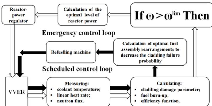
Fig. 1. The principal scheme of VVER FE cladding tightness control
